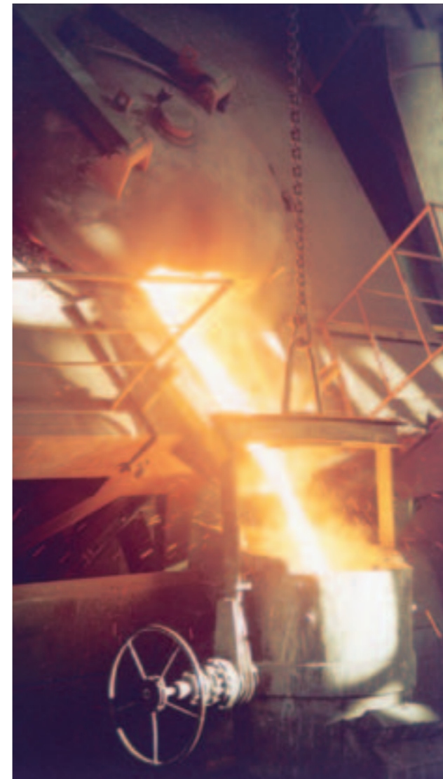
Cast from induction furnace
